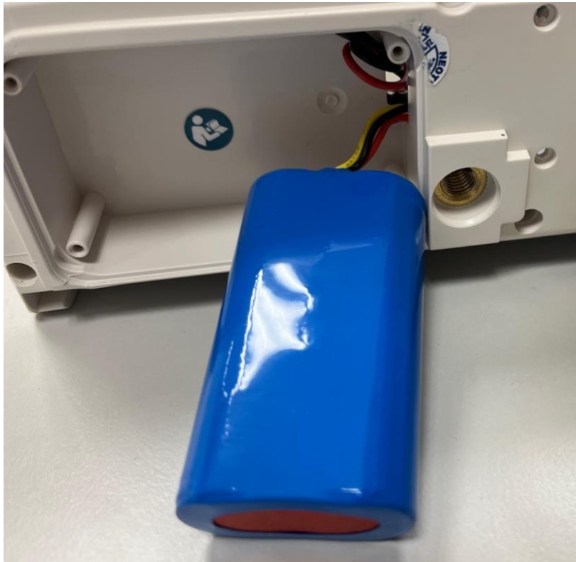
Internal battery of the MP-30 Syringe pump/MP-60 Infusion pump
