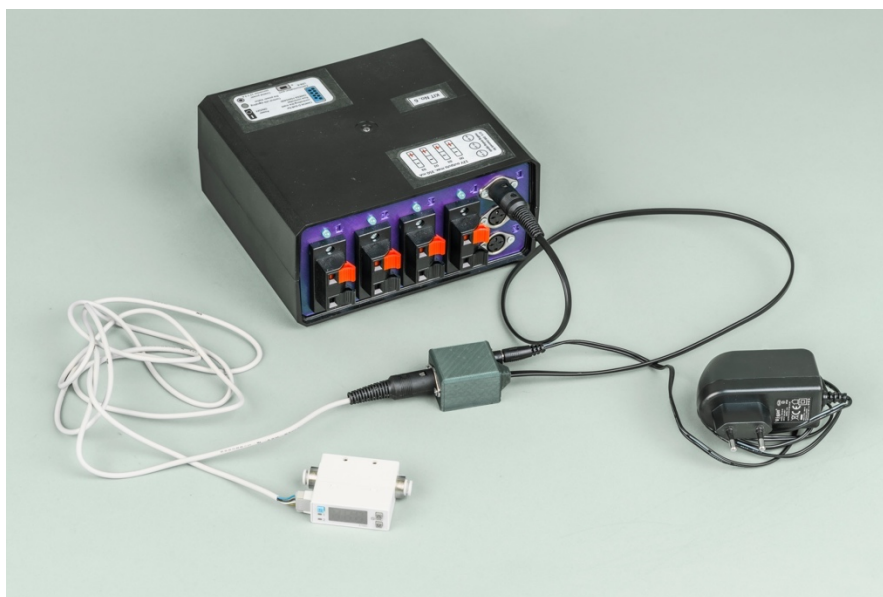
Fig. 31: 12V supply from Meluzína for measuring range of 0–50 L/min of the flowmeter or 24V supply from the distribution network for measuring range of 0–100 L/min.
