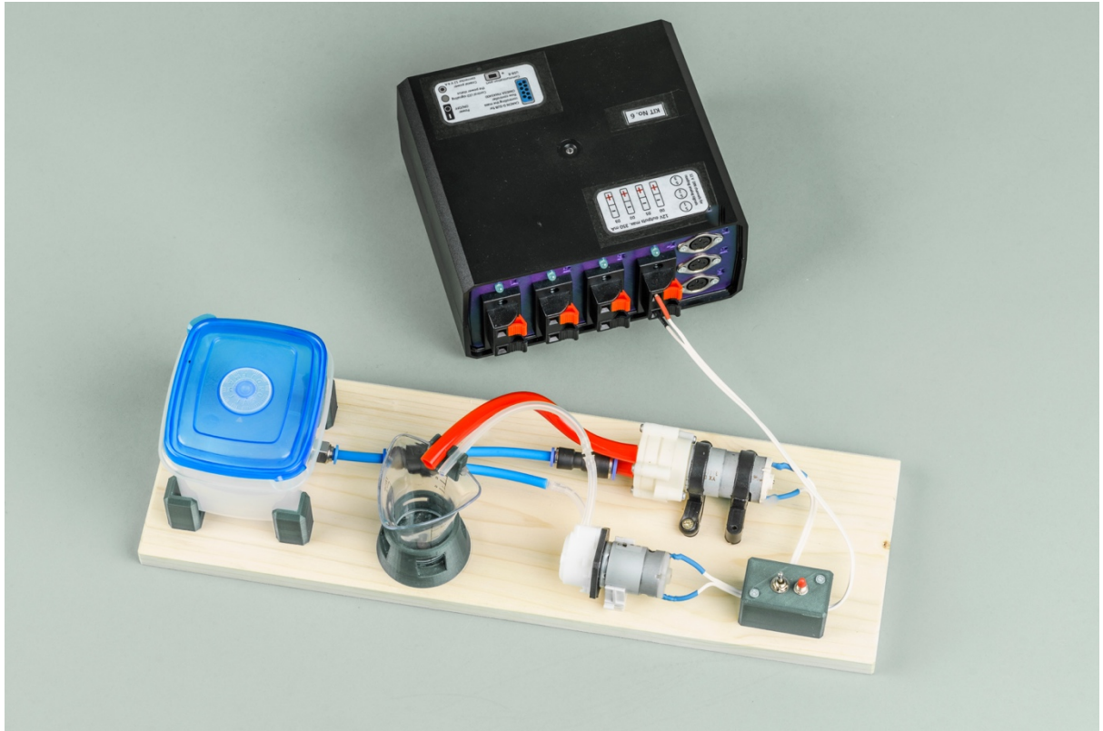
Fig. 74: Fully assembled apparatus of gear pump versus peristaltic pump
