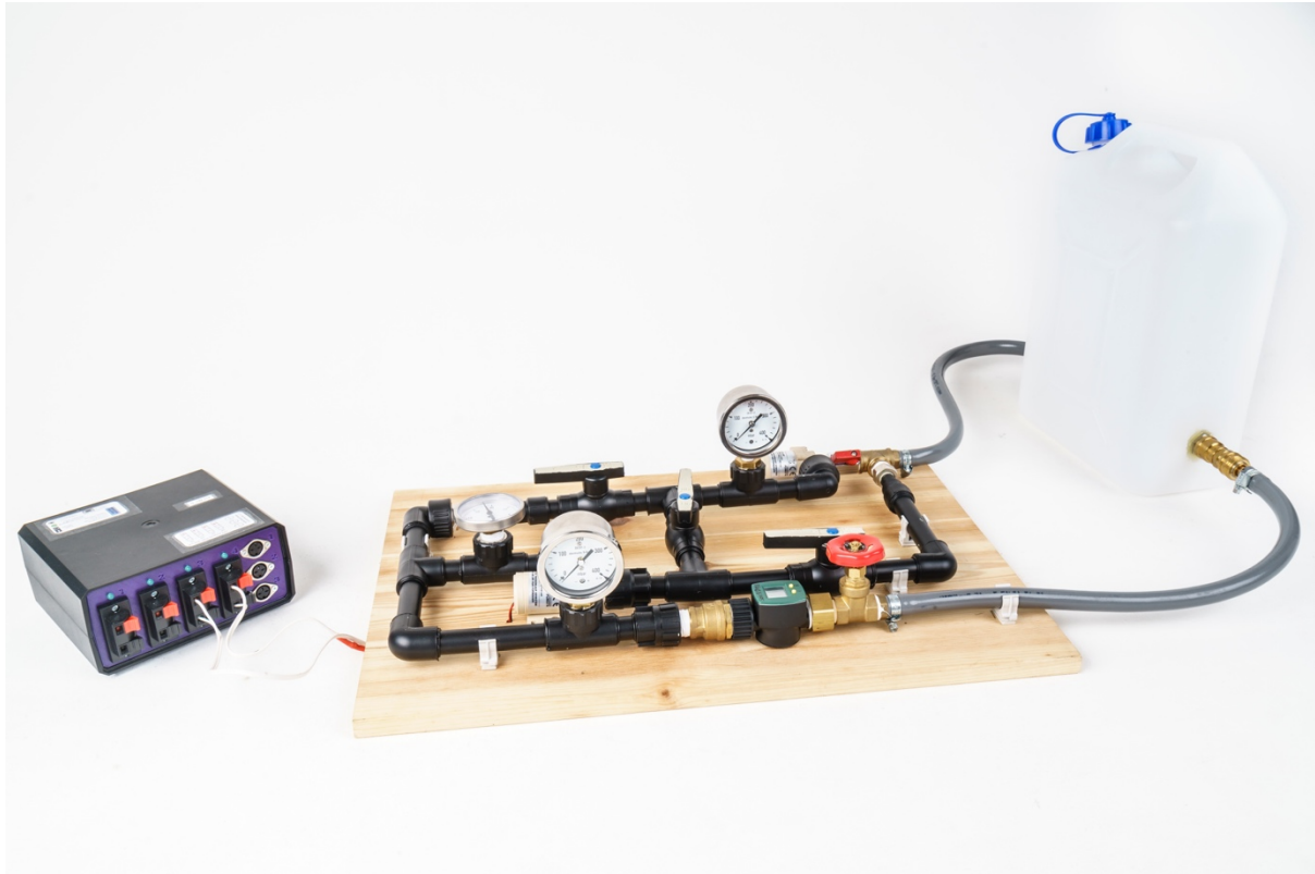
Fig. 73: Fully assembled centrifugal pumps apparatus
