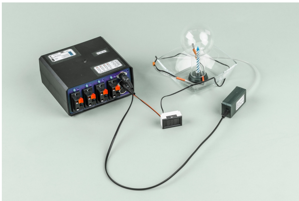
Fig. 51: A fully assembled water-candle experiment
