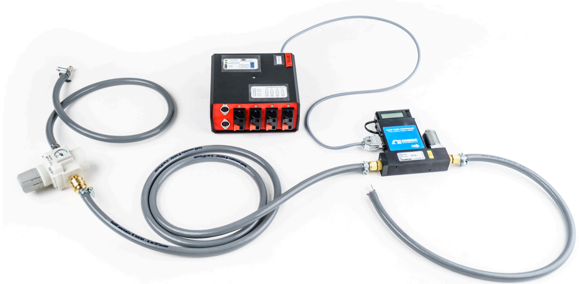
Fig. 13: Typical connecting to the air-distribution system
