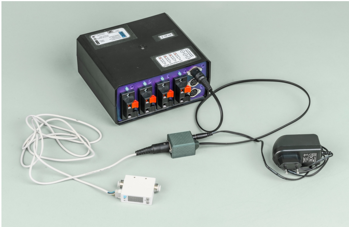
Fig. 30: 12V supply from Meluzína for measuring range of 0–50 L/min of the flowmeter or 24V supply from the distribution network for measuring range of 0–100 L/min.
