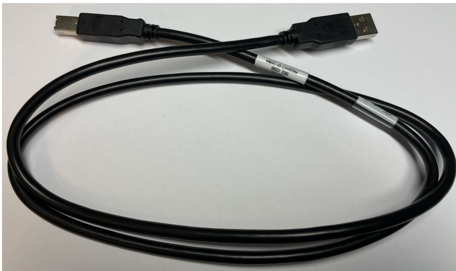
Fig. 8: Connector between Meluzína and PC – USB cable (male–male) type B – type A
