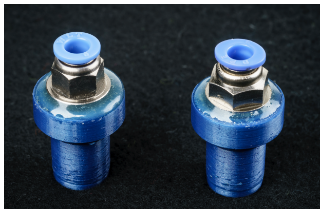
Fig. 44: An adapter between 6mm tube and 15mm I.D.
