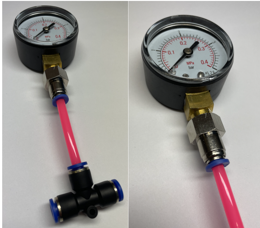
Fig. 39: 0–4 bar manometer and a typical connecting to the tubing
