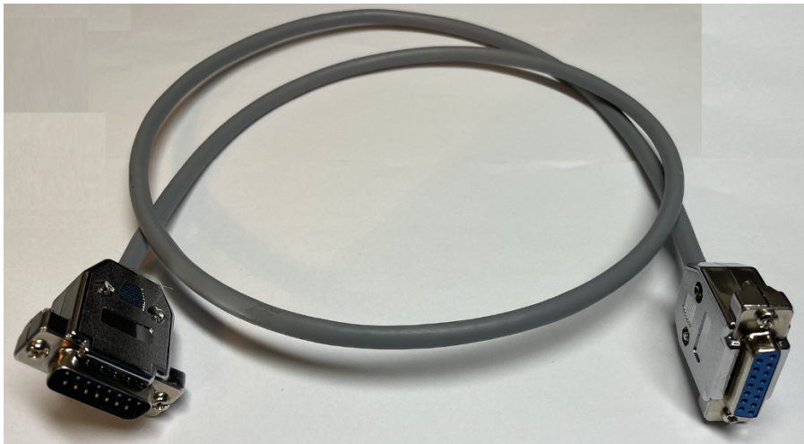
Fig. 7: Connector between Meluzína and OMEGA FMA5400 flow controller – 14 channel cable for communication
