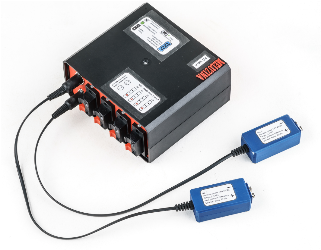
Fig. 25: Connection between Meluzína and two +/- 2kPa pressure sensors
