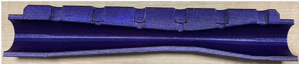
Fig. 64: Cross-section of the Venturi tube
