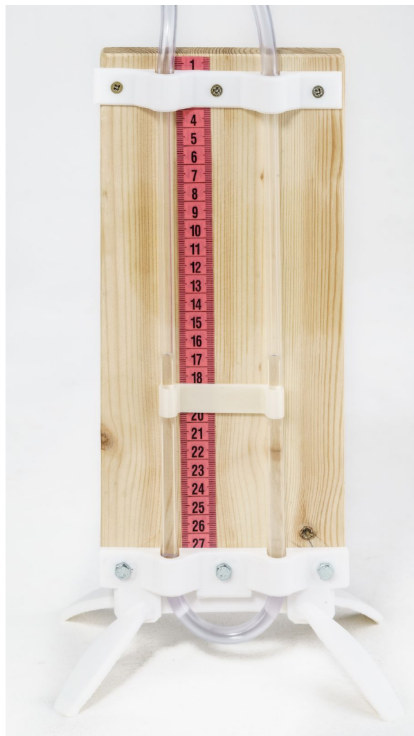
Fig. 74: A stand with capillaries for displaying the difference in levels during air flow
