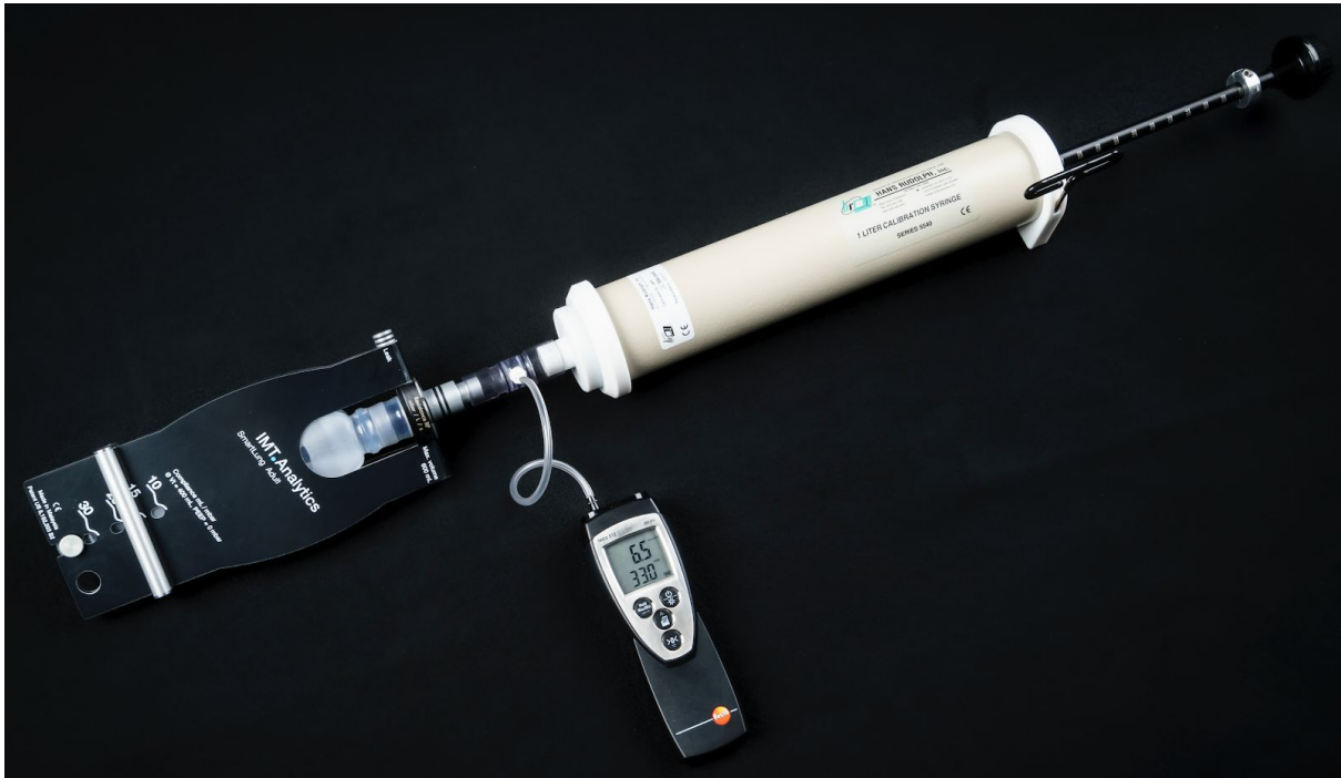
Fig. 47: Smartlung and the typical connection of the apparatus
