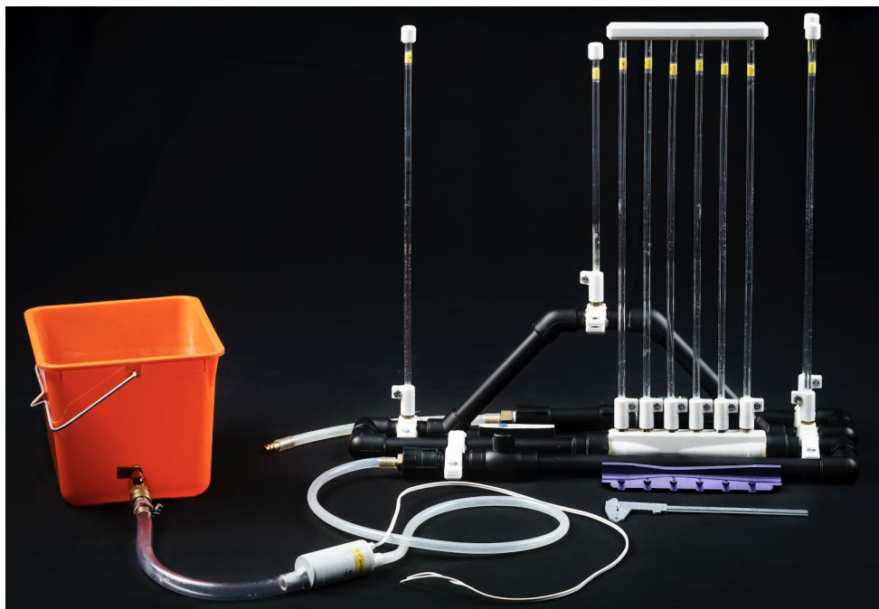
Fig. 68: The assembled apparatus with a water tank and a water pump
