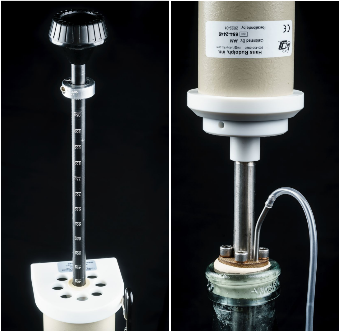
Fig. 46: A 1L calibration syringe and a connecting of a syringe to demijohn
