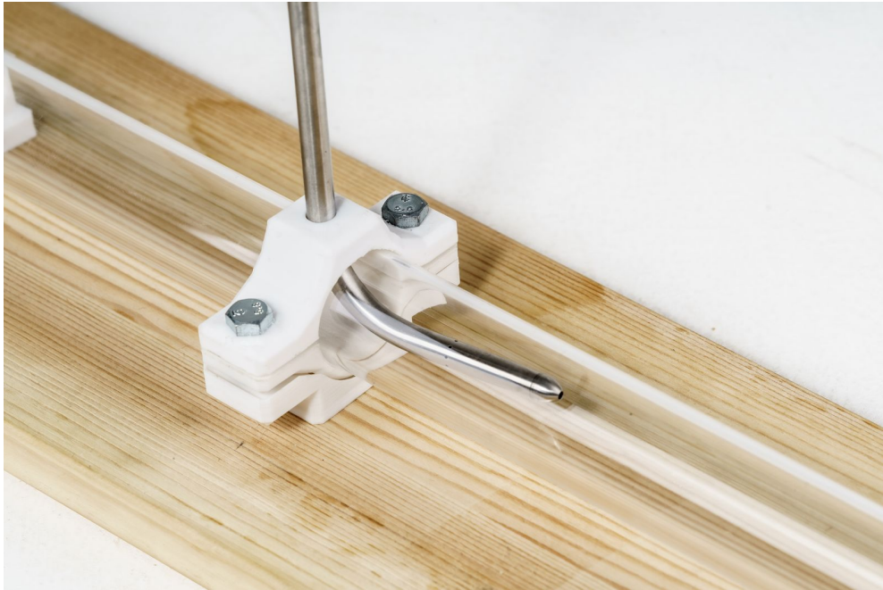
Fig. 73: Fixing the Pitot tube to the interior of the flow pipe
